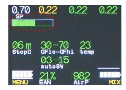
Soon absorbent in the bottom scrubber part is exhausted and starts cooling. This process is displayed on the sensor in the following way: the very left segment on the scale becomes brighter again.
