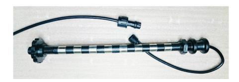
**Attention:** this system does not define CO2 level, it just measures temperature distribution in chemical absorbent layers (CO2 absorbent) in the scrubber starting from the first layer. Consequently, it does not give any signal if there is no absorbent in the system at all, or CO2 goes through scrubber due to damage or absence of O-ring. There will be no signal from this system if CO2 goes through valve box via either damaged, or absent non-return valve. THIS SYSTEM DOES NOT DEFINE CO2 LEVEL.
