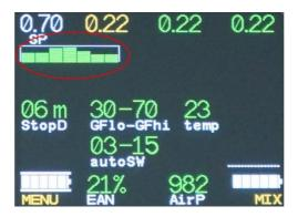
When operation time of he scrubber comes to an end, scrubber values will change in accordance with algorythm, namely: they will remind car fuel sensor, i.e. empty scale warns that it's not recommended to rely on the rebreather, and you should make emergency ascent as per Open Circuit mode.
