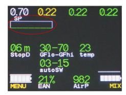
At the beginning the scale is displayed as an empty frame. Then as lower/bottom scrubber part is warming up, green segments will appear in the left scale part, then next segments to the right, and so on – from the left to the right. Segments' height is proportional to layer temperature (activeness).
