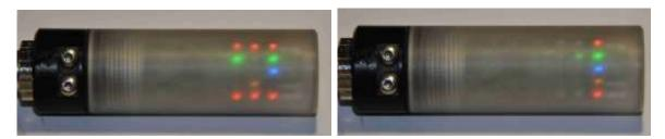
In case of choice of calibraton by oxygen figures 9 and 8 will alternatively flash.
