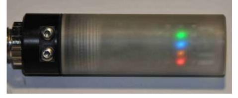
Replace the battery, if the charge level is lower than yellow LED.
