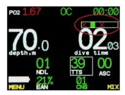
Eight gases' list is displayed in squares. Square number from left to right corresponds to the number of gas in the list. It is therefore convenient to have the list of gases from the deepest to the oxygen in the ascending order. In the example listed on a photo three active OC gases are numbered 1, 3, and 5.
