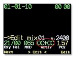
Navigating between fields is made with → button, changing the field value is made with + button. MOD field value is taken into account when best mix is offered at the moment of gas change via ->selectmix menu item, and when TTS value calculation and when planning your dive.
