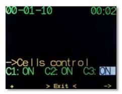
• With at least one Oxygen cell activated, AV1 will automatically offer to calibrate.
