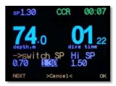
manual switching between Low, High and Deco Setpoints. Choose the required Setpoint with button *Next* and confirm with button *OK*.
