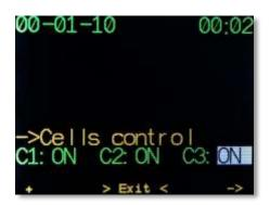
AV1 in CCR mode can control  $PO_2$  in the loop by means of one, two or three Oxygen cells of R22, R17 or similar type. Quantity and cell number is set in this menu. See in detail - **PO2** Cells Control.
