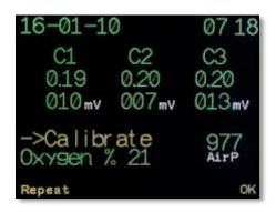
When calibration is finished, press **OK** to save, or, if required press **Repeat** to repeat.
