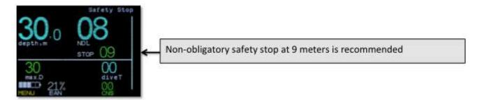
When reaching the safety stop depth, safety stop countdown timer will automatically swith on.
