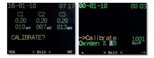
If cells show the same stable values within 10 seconds and are within the same working range, the cells will be automatically calibrated. Otherwise, the cell (cells) will be switched off **OFF** mode.
