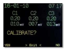
Start of calibration of connected Oxygen cells.
