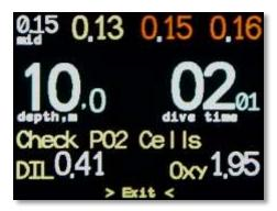
PO2 values at the current depth are displayed at the bottom of AV1 screen in case of flushing the loop with diluent or (up to 10 meters inclusive) with oxygen. The function works on all AV1 products in **CCR** mode.
