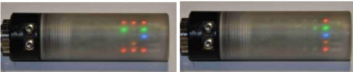
In case of choice of calibration by oxygen figures 9 and 8 will alternatively flash.
