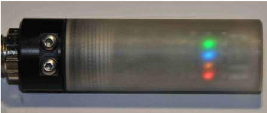
Replace the battery, if the charge level is lower than yellow LED.
